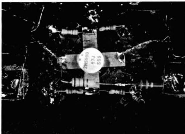
Underside of amplifier. Emitter-resistor assembly is shown paralleled between emitter tabs and ground plane. Input and output transformers are at extreme right and left.
