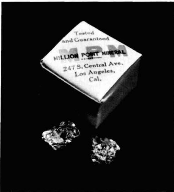
Steel galena crystal offered to amateurs in the 1920s.
